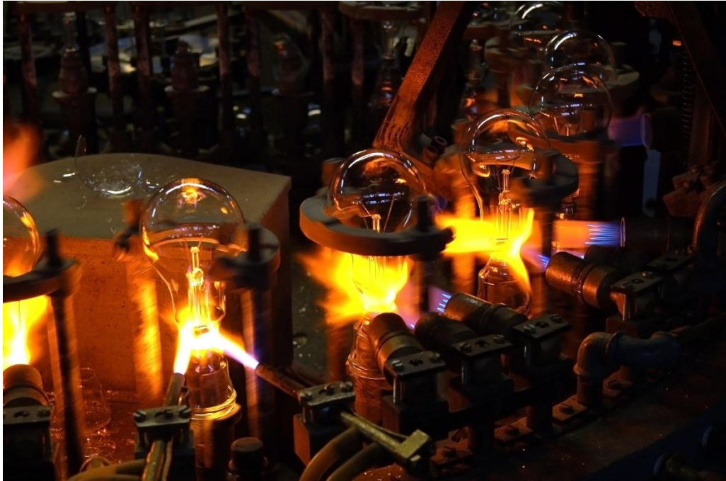
Mass flow controllers in Glass Manufacturing and processing deliver precise gas mixtures for the burners.
