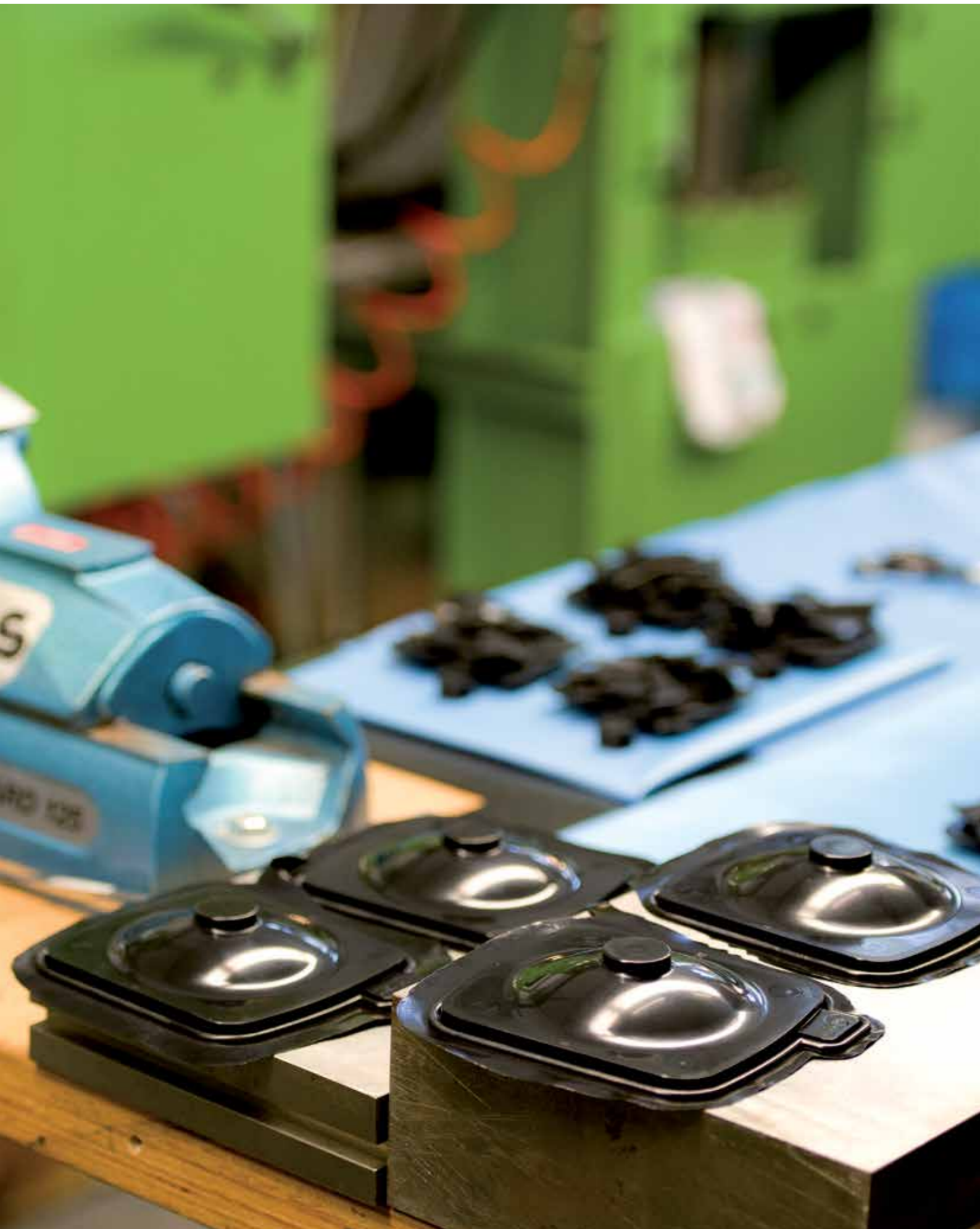
Diaphragm after vulcanisation, prior to trimming.
