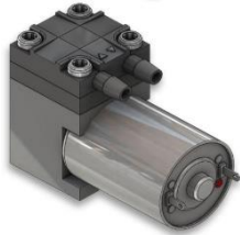
SP 270 EC-LG-L Eccentric Diaphragm Pumps for Liquids Free flow rate: 100 ml/min Max pressure: 14.5 psi / 10.0 m H2O Max suction height dry (priming): -4.35 psi / -300 mbar Max suction height filled: -3.0 m H2O
