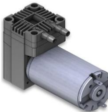
SP 620 EC-L Eccentric Diaphragm Pumps for Liquids Free flow rate: 710 ml/min Max pressure: 21.7 psi / 15.0 m H2O Max suction height dry (priming): -8.7 psi / -600 mbar Max suction height filled: -9.0 m H2O
