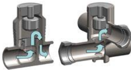
Fig. 2: Internal media flows in the case of a standard valve body (left) and modular body
